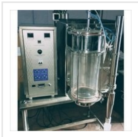
LSD 01 Laboratory Spray Dryer
